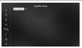
If the surround back speakers are not used in the main zone, their surround back amplifier channels could be assigned for Back, Height 1, Height 2, Zone 2 and Front (Bi-Amp) use.
