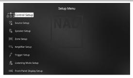
The Setup Menu allows one to customize the operation of the T 758 to the ancillary equipment used in one's specific AV system. Unless your system exactly matches the factory defaults as shown in the accompanying Quick Start Guide, you will need to use the setup menu to configure the inputs of the T 758.
