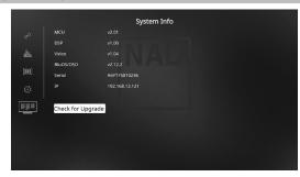
"System Info" displays information about the loaded firmware and BluOS versions, serial number and IP address.
