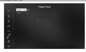
The T 758 features a configurable  $\pm 12$ V TRIGGER OUT that can be used to activate a component or system it is fed into. It is used to turn on/off other compliant devices.
