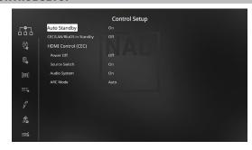
The T 758 supports HDMI Control (CEC) and Audio Return Channel (ARC) functions. Both functions are possible if external devices that also support both features are interconnected with the T 758 via HDMI connection.
