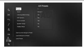
The T 758's simple but powerfully flexible system of "A/V Presets" allows you to customize virtually every aspect of your audio-video playback, and recall them with a single key-press. The parameters "Listening Mode", "DSP Options" and "Tone Controls" accessible via the "Main Menu" together with "Speaker Setup" and "Display Setup" configurable through "Setup Menu" are stored together as a single A/V Preset.
