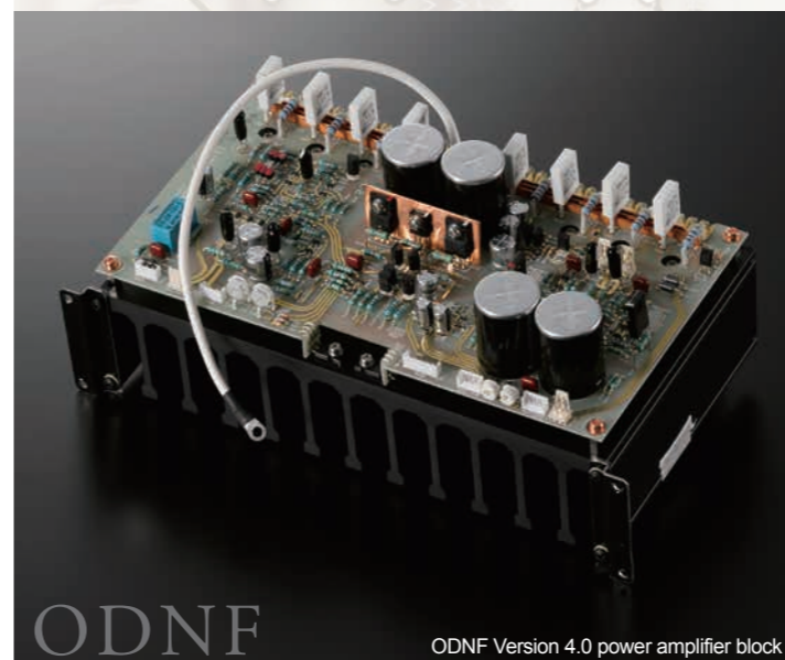
ODNF Version 4.0 power amplifier block
