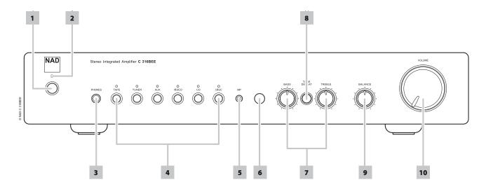
1 STANDBY: With the rear panel POWER switch set to ON position, press this button to switch ON the C 316BEE from standby mode. The Standby LED indicator will turn from amber to blue. Pressing the STANDBY button again turns the unit back to standby mode.
