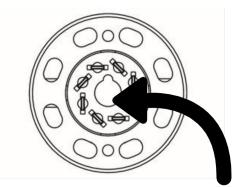
Some tubes, including the 5AR4 rectifier tubes in your EvoLotion Series Preamplifier, have a "center locating key" which must line up with the socket! If you misalign them and use brute force to push the tube in place, you will damage important and expensive parts of your preamplifier! This damage will void your warranty so use caution when installing power tubes!
