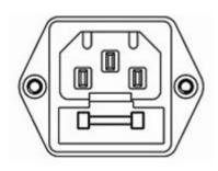
Mains Fuse: The mains fuse is located on the rear of the amplifier, just below the power cord socket (see picture on the left). The fuse rating is 1 x Littelfuse 213 Series 1A Slow Blow 5 x 20mm fuse for 100-125VAC and Littelfuse 213 Series 0.5A (500mA) Slow Blow 5 x 20mm fuse for 200-250VAC. Always replace with the same type and value fuse! The fuse holder can be opened using a small slotted flat blade screwdriver.
