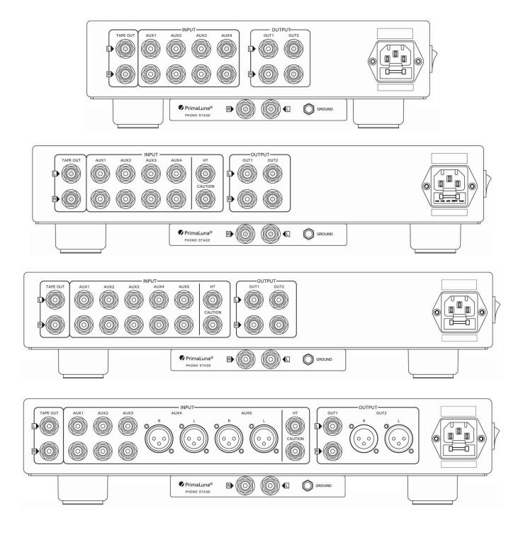
At the rear panel, you will find your inputs including the HT pass-through, Tape Out, and Preamp Outputs.
